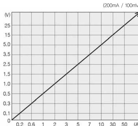
• Condition : the output voltage measured in increased current by attaching the ZCT impedance ( $2\Omega$ ) to secondary ZCT
