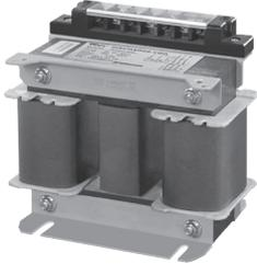
The discharge coil for the low voltage static capacitor is the discharge coil for the capacitor used for the purpose of the short-term discharge to control the overvoltage generated from the fast automatic control re-input due to the residual charge remaining in the condenser when opening the condenser from the circuit and to secure the safety on the human contact.
